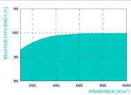
Typical module performance under low irradiance conditions in comparison to STC conditions ( $25\,^{\circ}\text{C}$ ,  $1000\,\text{W/m}^2$ ).
